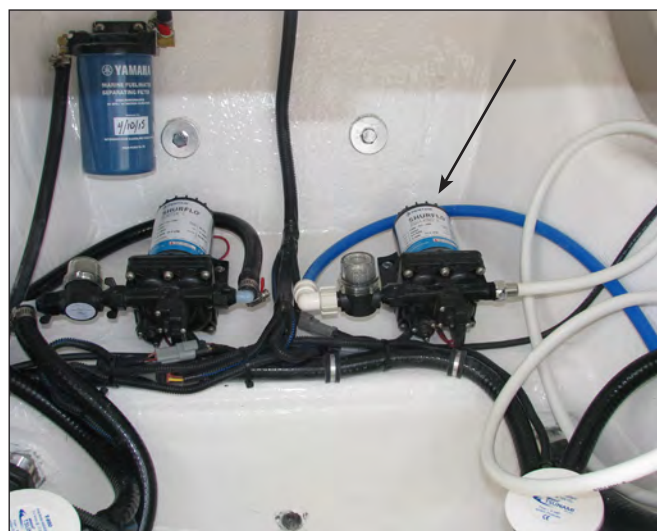
Fresh & Raw Water Pump Location In Stern Bilge
