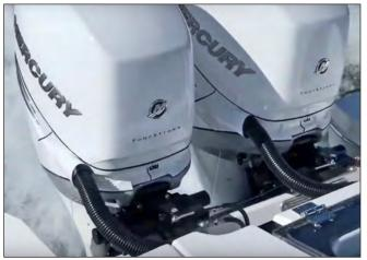
Mercury Engines With Electronic Steering
