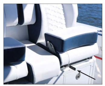
Helm Seat Slide Track Lock Release Lever
