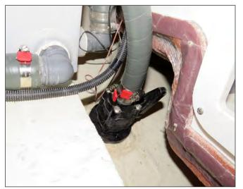
Waste Overboard Discharge Thru-Hull Valve
