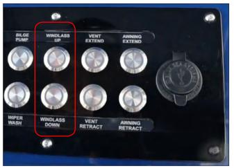
Windlass Switches In Helm Switch Panel
