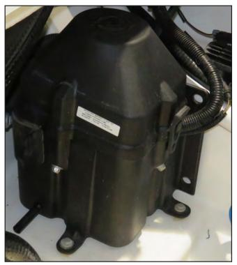
Typical Mercury Steering System Power Assist Pump
