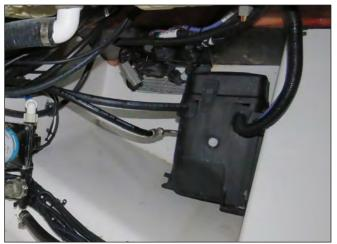
Typical Mercury Electronic Steering Pump
