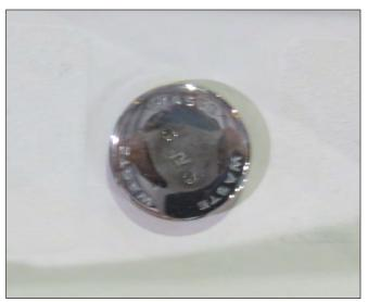
Holding Tank Waste Deck Pump Out Fitting
