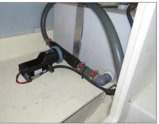
Waste Overboard Discharge Pump & Holding Tank
