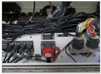
**Electronics Main Bypass Switch**
