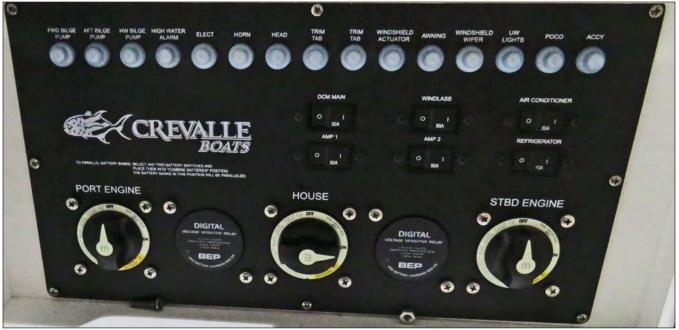
Battery Switch Panel, Battery Switches, Main Circuit Breakers & Accessory Breakers
