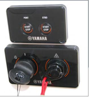
Typical Twin Engine Yamaha Command Link Ignition & Engine START/STOP Switch System
