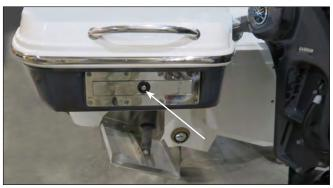
Ladder Latch Release Button & Ladder Retracted In Compartment
