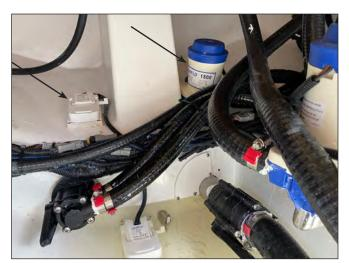
Emergency Bilge Pump & Emergency Pump & Alarm Automatic Switch
