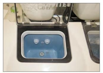
Aft Livewell Drain Fitting, Light & Overflow/Fill Valves
