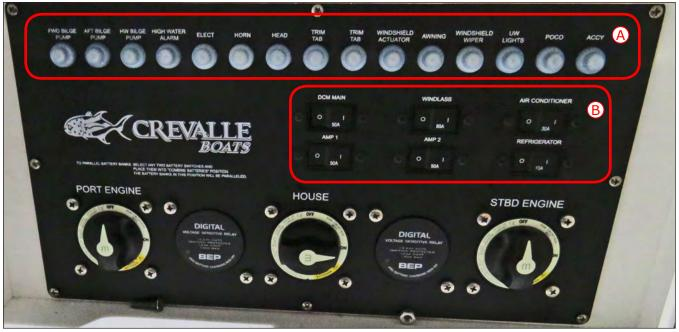
Accessory & Main Circuit Breakers In Battery Switch Panel
