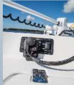
Note: All 24 SE boats come pre-rigged for your dealer to easily install a trolling motor. Trolling motor panel includes an outboard trim switch and Deltran Battery Tender Trolling Motor receptacle.
